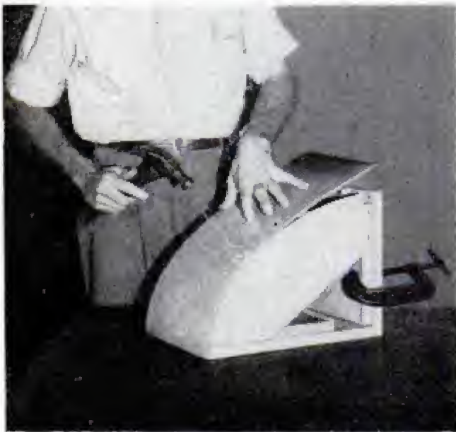
Above, compartment frontpiece is glued and nailed in place with brads. Heads are set below surface and holes filled. Below, after bandsawing to contour and applying facing, bottom frame is nailed to shelf
